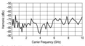
Typical 2nd harmonic levels measured at output power of +6 dBm  $\,$
