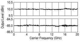
Typical output level accuracy and flatness at +10 and -85 dBm
