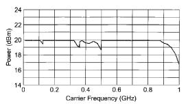
Typical maximum available output power from 0.01 to 1 GHz at 25°C
