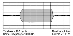
Typical pulse modulation envelope illustrates the fast rise and fall times, excellent flatness, and pulse fidelity of the 83731B/83732B.
