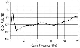
Typical pulse modulation on/off ratio at +8 dBm
