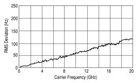
Typical residual FM measured in 50 Hz to 15 kHz bandwidth, CW mode, with high-stability timebase, Option 1E5
